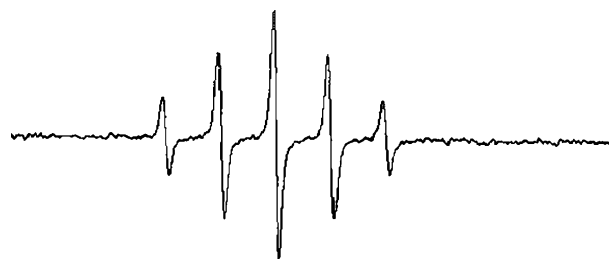
Scheme 3. ESR spectrum of 6g at 10^{-5} mol/L in phosphate buffer (pH 7.4).
